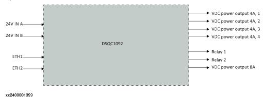
The four VDC power outputs which provide 4A, can be connected in parallel. This to provide other combinations such as 2x8 A or 1x16 A configurations.
